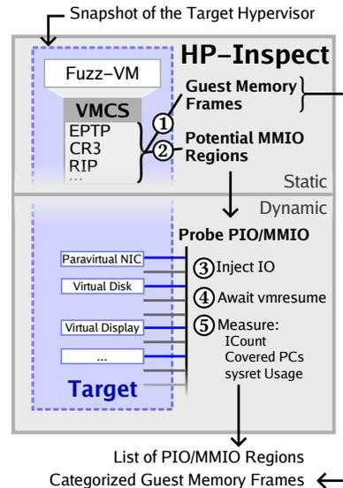
Figure 3: HYPERPILL-Inspect analyzes the hypervisor’s PIO/MMIO/Memory input-space.
