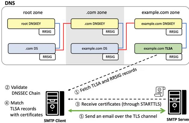
**Figure 1:** Overview of how DANE works along with DNSSEC and STARTTLS. The integrity and authenticity of TLSA records are supported through DNSSEC chain validation; Each RRSIG is the signature of a record set (e.g., TLSA records) verified with a DNSKEY (blue lines) and each DS record is updated by a child zone (red lines). After DNSSEC chain verification, the SMTP client verifies the obtained certificate by matching with it to a TLSA record.
