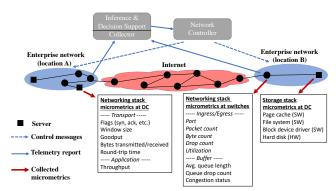
Figure 1: **High-level MicroMon Design.** Figure shows the integration of our HW and SW micro-metrics collection and dissemination in MicroMon.
