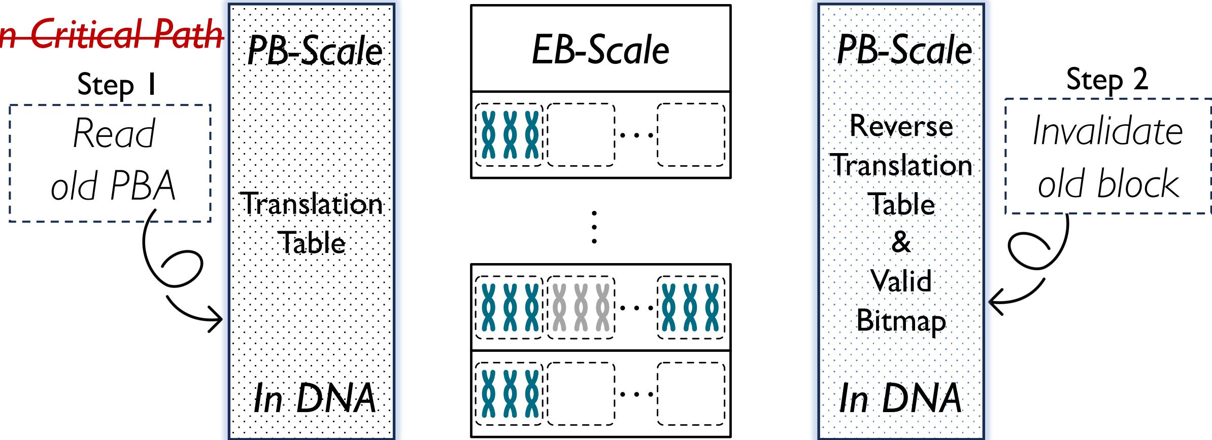
Delay invalidation to block read operation
