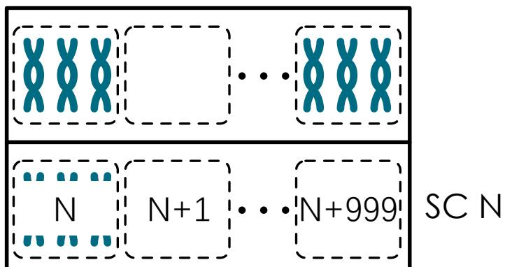
Assigning Physical Block Address to each block (PBA)
