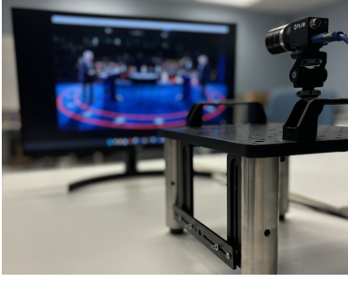
Figure 5: A visualization of one of our experimental setups where a camera is focused on a display.
