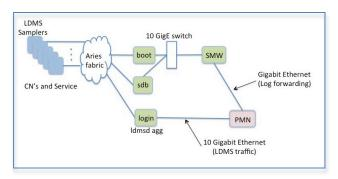
Figure 5 illustrates the Application Readiness Testbed (ART) system monitoring configuration
