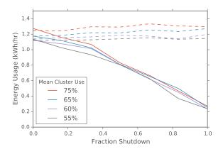
Figure 7: Energy usage of test cluster during partial shutdown experiments. Solid lines indicate power usage during the shutdown, while dashed lines indicate power usage during full operation.
