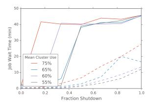
Figure 8: Maximum (solid) and mean (dashed) job wait times during partial shutdown experiments.
