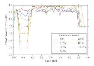
Figure 6: Total power consumed during experiments where variable numbers of machines were shut down during simulated peak pricing.
