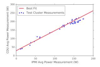
Figure 5: Comparison between node level IPMI measurements and rack level CDU measurements. Best fit shows the model relationship used to convert IPMI data to estimated total power draw.
