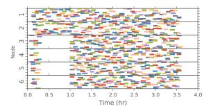
Figure 3: Diagram of job scheduling during a four node temporary shutdown experiment. Each colored rectangle displays the execution of a single LAMPPS test job running for approximately 5 minutes.
