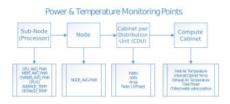
Figure 2: Energy measurement systems in EDEALS.
