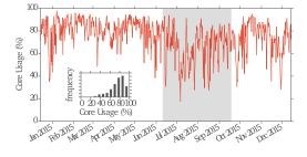
Figure 1: Average core usage for a 244 node shared HPC partition in the Midway cluster. Note that the period of peak energy demand (gray background) coincides with a period of reduced core usage. Insert shows usage statistics histogram.
