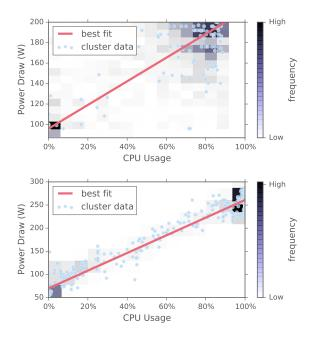
Figure 4: Power data for test cluster (top) and production cluster (bottom) nodes in presence of variable usage. The slope and intercept of the line are used to determine  $u_v$  and  $u_0$  respectively.
