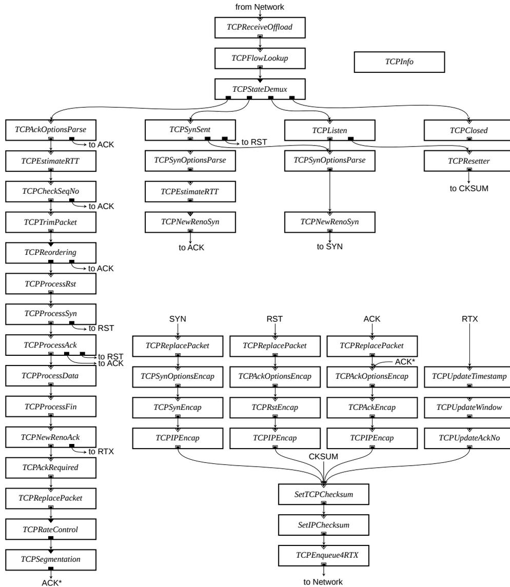
Figure 2: cTCP configuration for incoming network packets.
