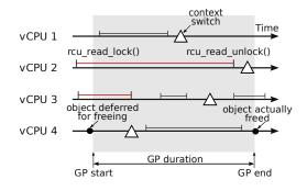
Figure 1: Linux-kernel grace period (GP). Red critical sections marked might hold references to the deferred object.
