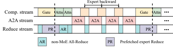
Figure 9: Pipeline scheduling of streams in backward pass.
