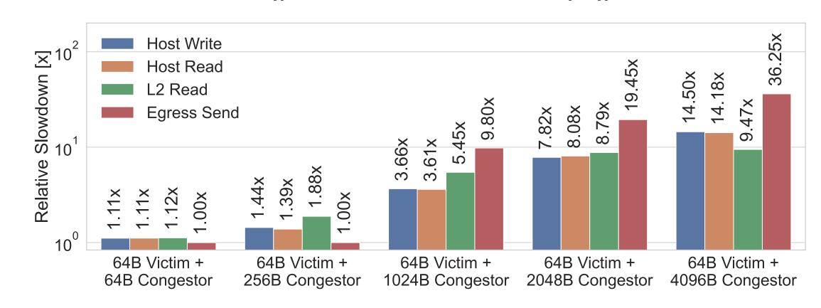
FIFO processing of DMA requests results in HoL-blocking
