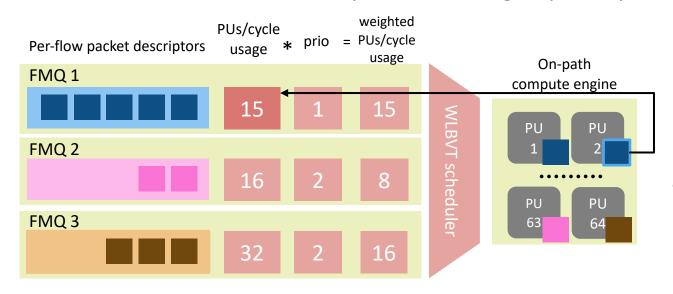
System state at cycle N + 2: Feedback update to FMQ 1 PU usage
