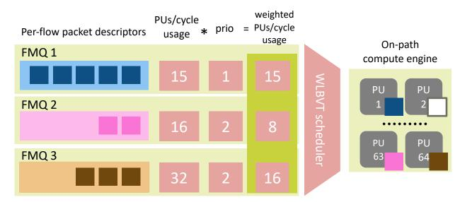
System state at cycle N + 3: Find FMQ with minimal PU usage
