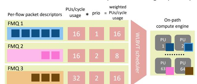
System state at cycle N + 1: PU 2 finishes processing FMQ 1 packet
