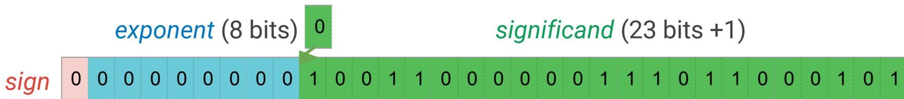
$$\text{Value} = (-1)^{\text{sign}} \times \text{significand} \times 2^{(\text{exponent} - \text{bias})}$$
