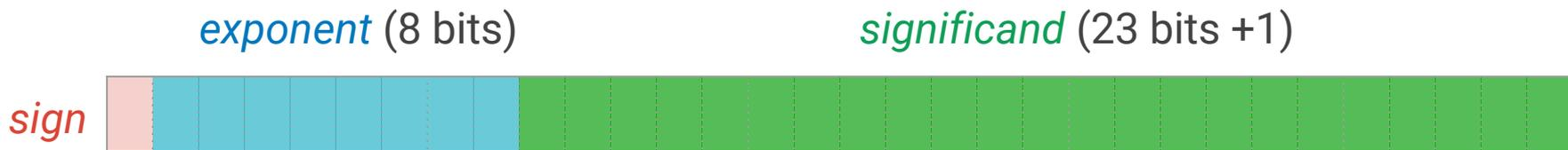
$$\text{Value} = (-1)^{\text{sign}} \times \text{significand} \times 2^{(\text{exponent} - \text{bias})}$$
