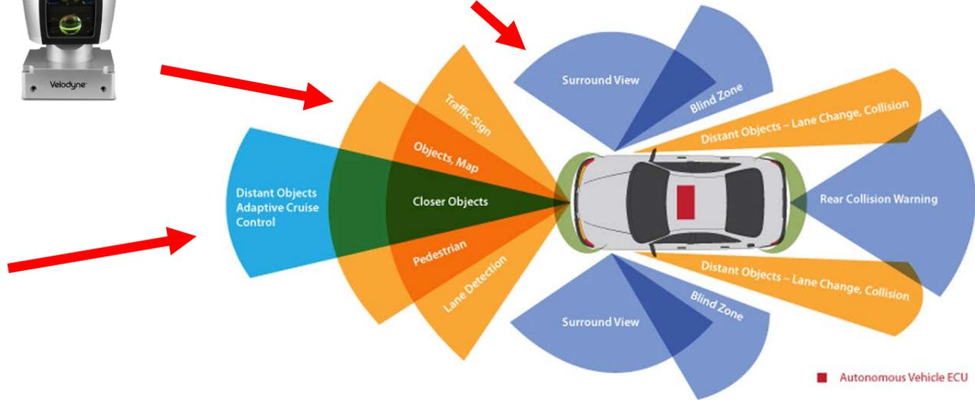
■ Long Range RADARs ■ LiDAR, SRR ■ Camera - Stereo, Monocular ■ Ultrasonic Sensors
