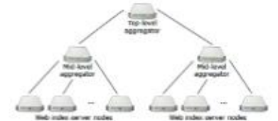
Figure 1: Architecture of index serving system of Web search engine with two aggregation levels (MLA and TLA). The user query is processed on index servers, which send responses to MLAs, which send aggregated responses to TLA.
